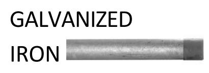
A dull, silver colored pipe that is hard to scratch with a coin or key. Scratching leaves a dull gray color. A magnet <u>WILL</u> stick to a galvanized iron pipe.
