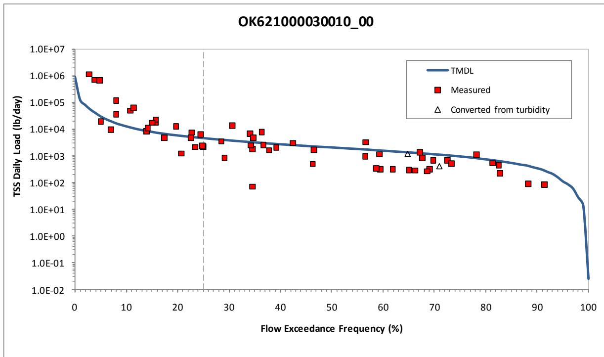
**Figure 5-84 Load Duration Curve for Total Suspended Solids in Deer Creek
