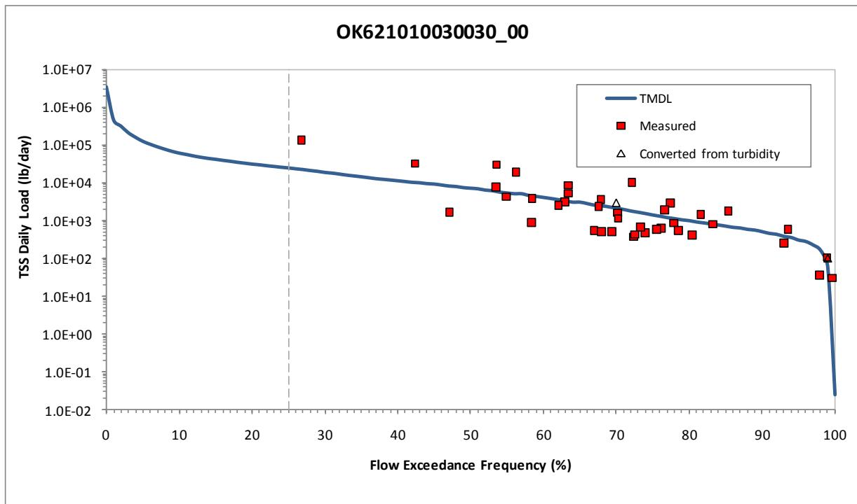
**Figure 5-92 Load Duration Curve for Total Suspended Solids in Chikaskia River,
