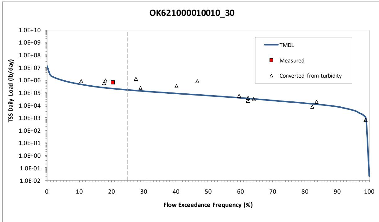
**Figure 5-83 Load Duration Curve for Total Suspended Solids in Bois d'Arc Creek
