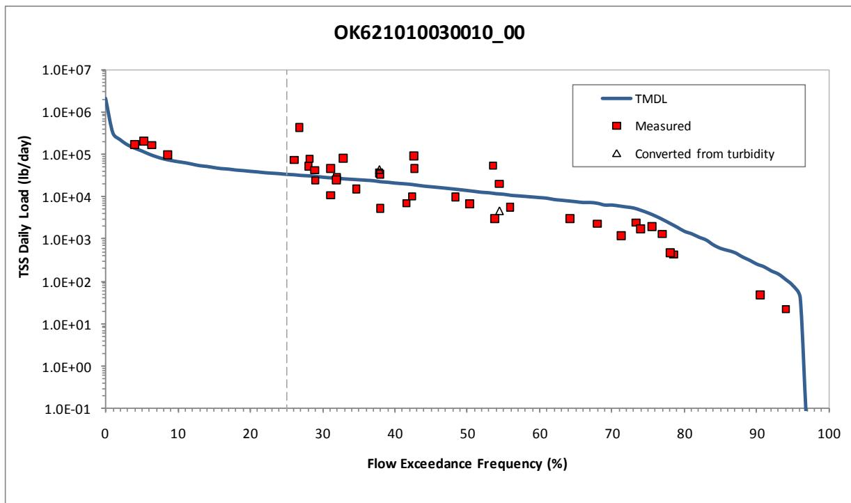
**Figure 5-91 Load Duration Curve for Total Suspended Solids in Driftwood Creek
