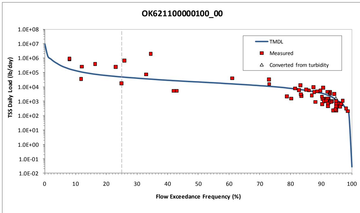
**Figure 5-95 Load Duration Curve for Total Suspended Solids in the Arkansas River
