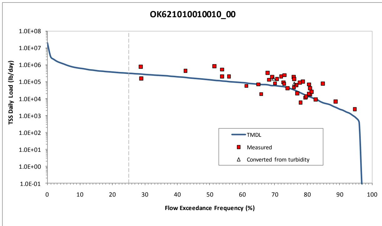
**Figure 5-88 Load Duration Curve for Total Suspended Solids in Arkansas River, Salt Fork (OK621010010160\_00)**
