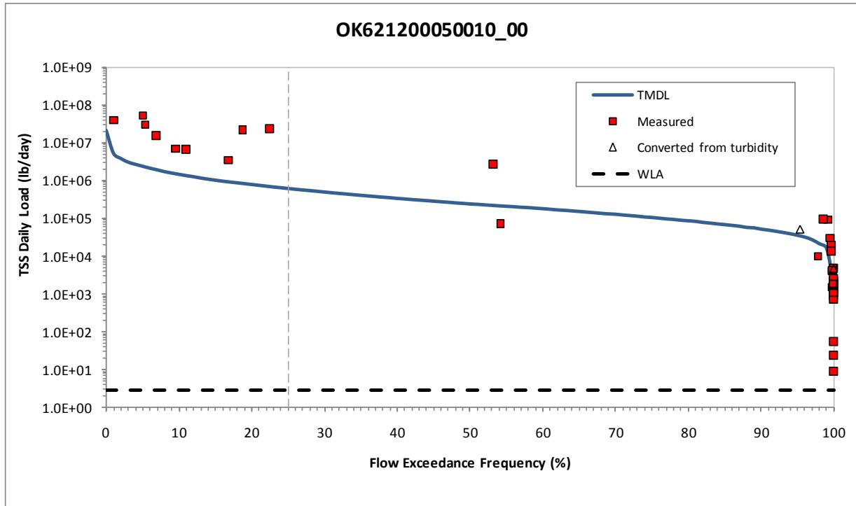
**Figure 5-97 Load Duration Curve for Total Suspended Solids in Red Rock Creek, Upper (OK621200050010\_10)**
