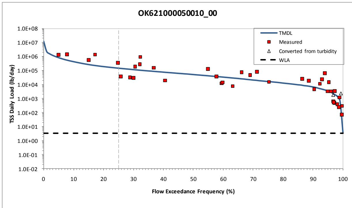
**Figure 5-86 Load Duration Curve for Total Suspended Solids in Crooked Creek
