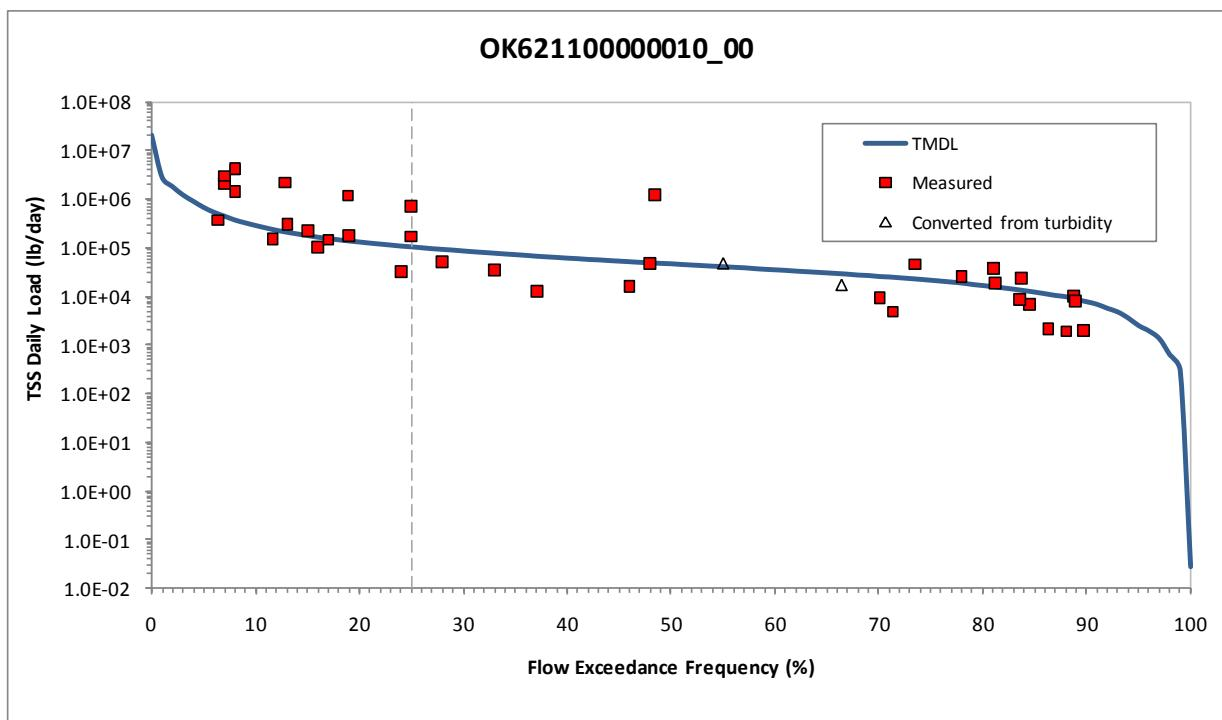
**Figure 5-93 Load Duration Curve for Total Suspended Solids in Chikaskia River, Upper (OK621100000010\_10)**
