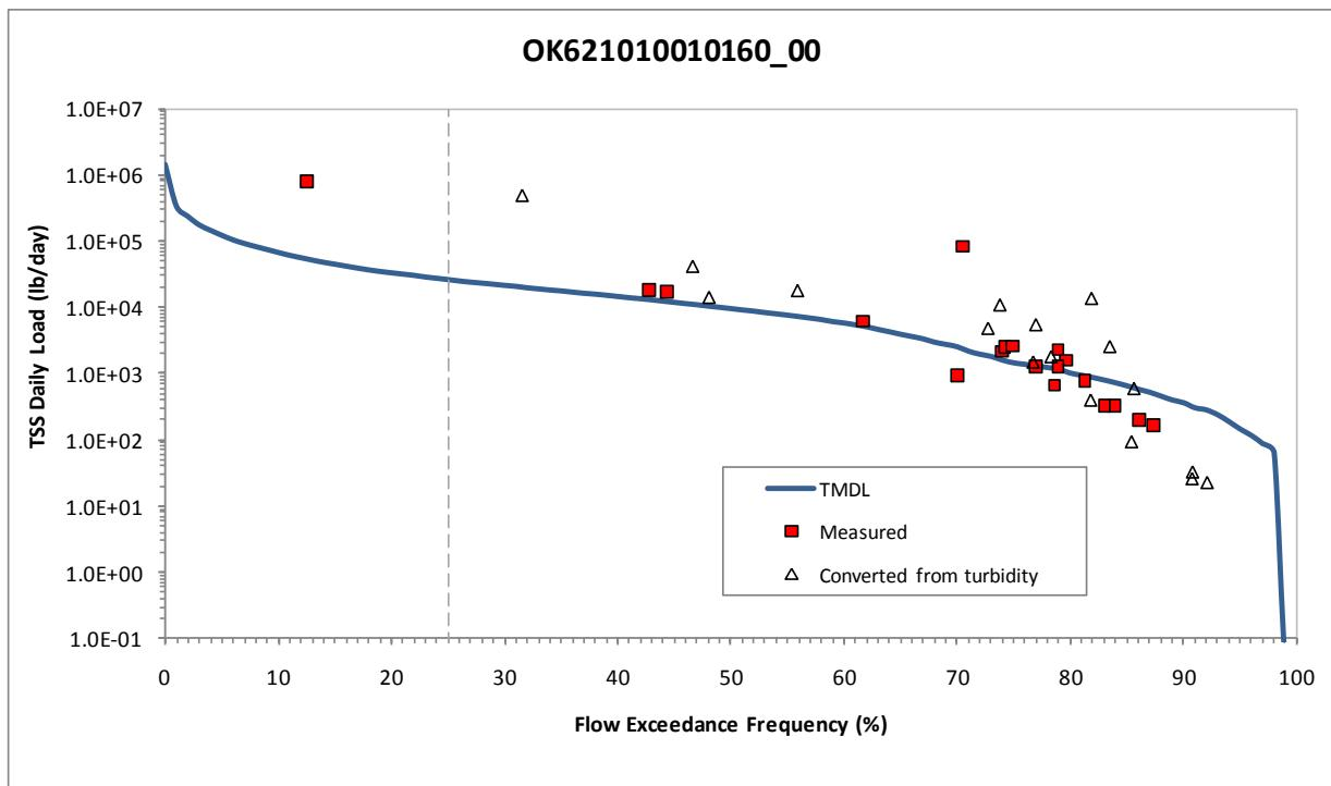
**Figure 5-89 Load Duration Curve for Total Suspended Solids in Turkey Creek
