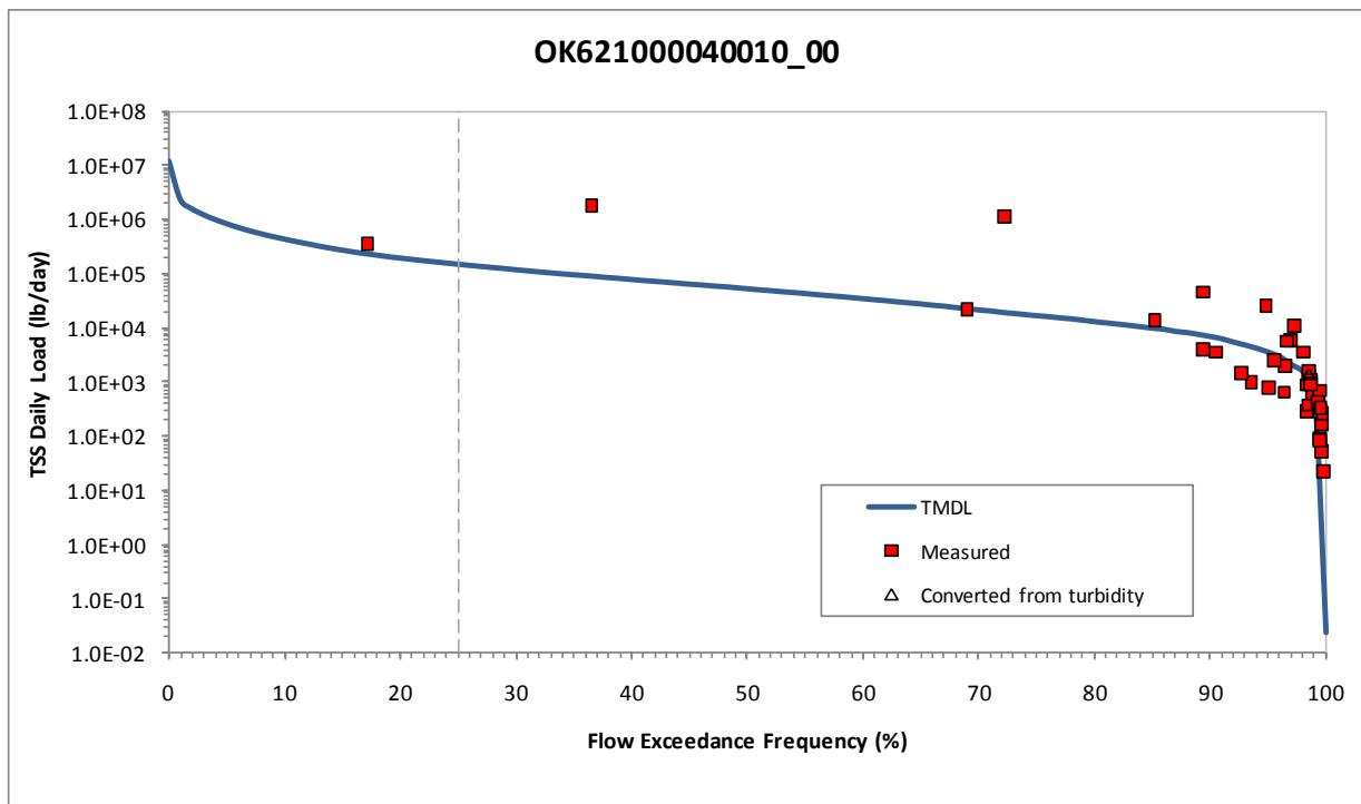
**Figure 5-85 Load Duration Curve for Total Suspended Solids in Pond Creek
