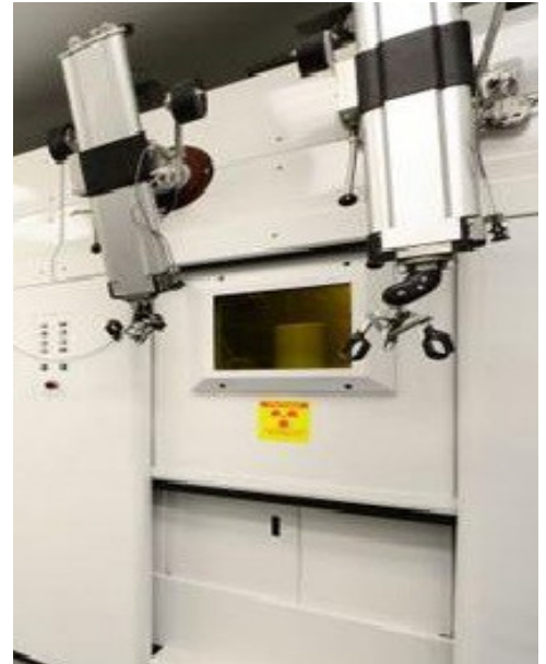
Figure F-1 Example of a hot cell with remote manipulators
