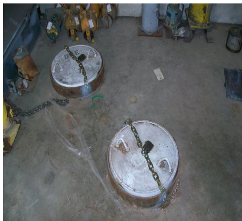
Figure G-2 Examples of source down-hole storage
