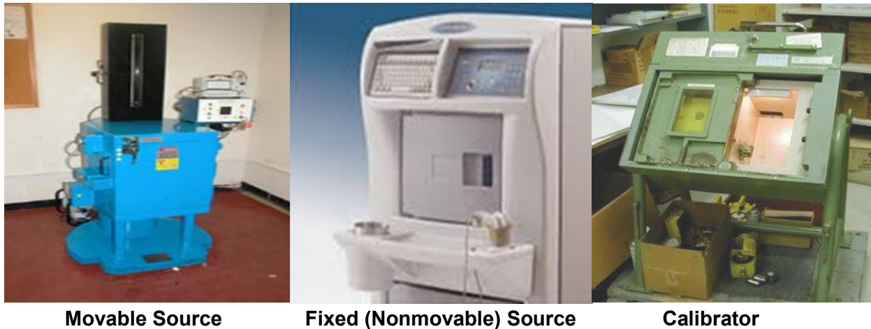
Figure C-1 Examples of self-shielded irradiators
