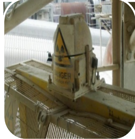
Figure D-1 Example of a fixed gauge
