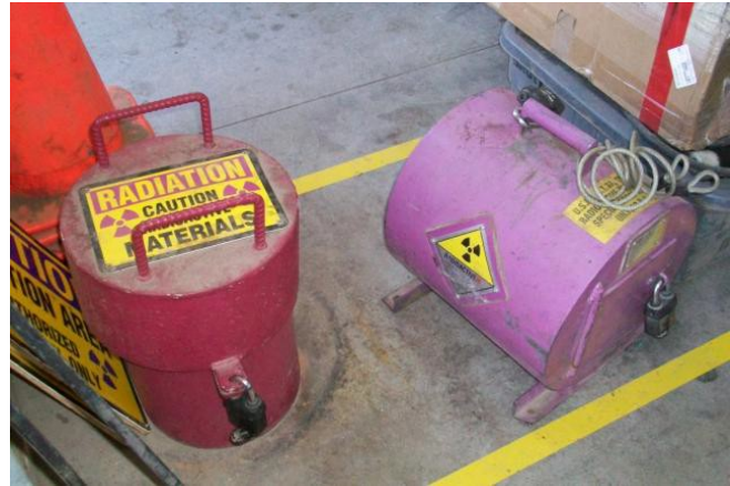
Figure G-1 Well logging source transport containers
