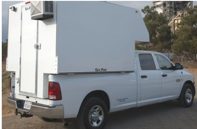
Figure H-2 Secured radiography darkroom truck
