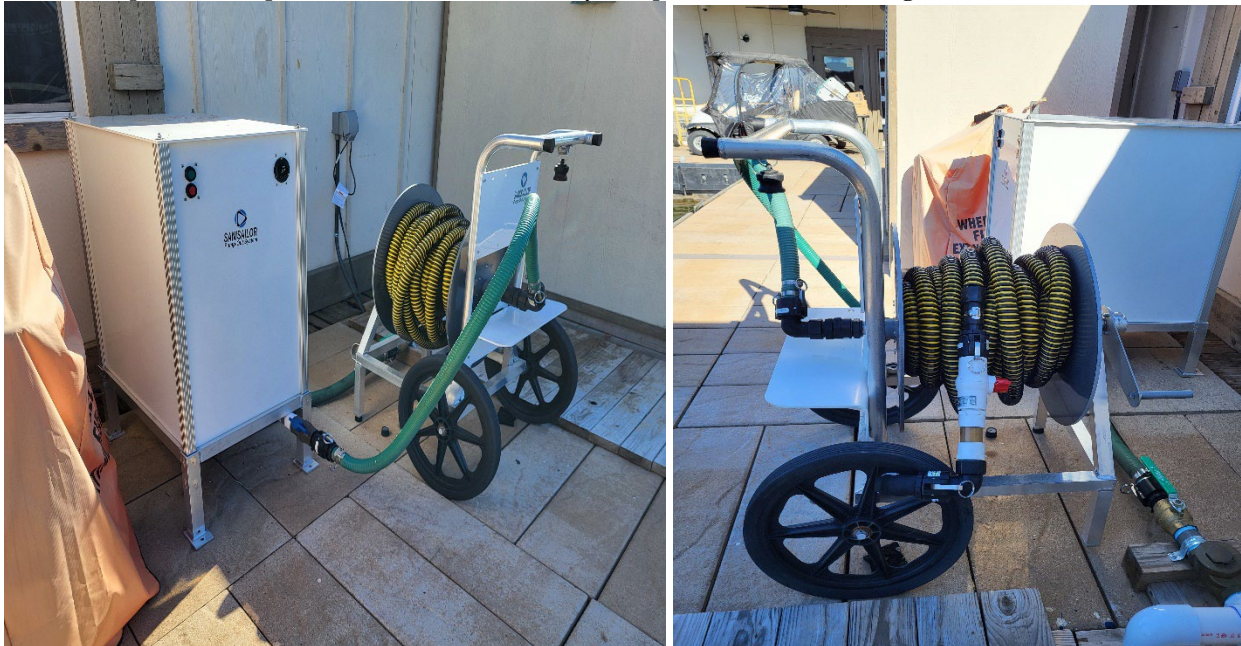
Photo Series #3. Keystone Harbor Marina. February 14, 2024 Mobile Pump-out station placed for boats to dock close by to deposit their onboard sewage.
