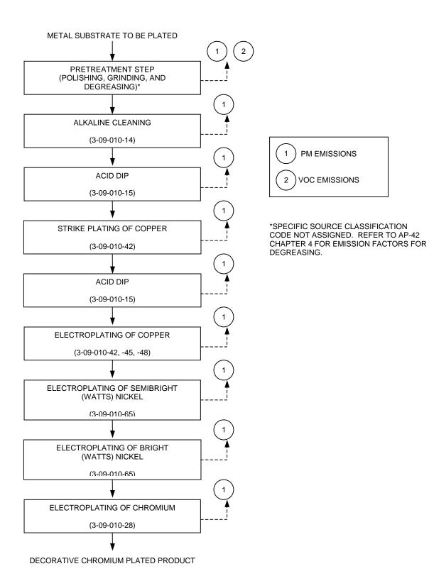
Figure 12.20-2. Flow Diagram for decorative chromium plating on a metal substrate. (Source Classification Codes in parentheses.)
